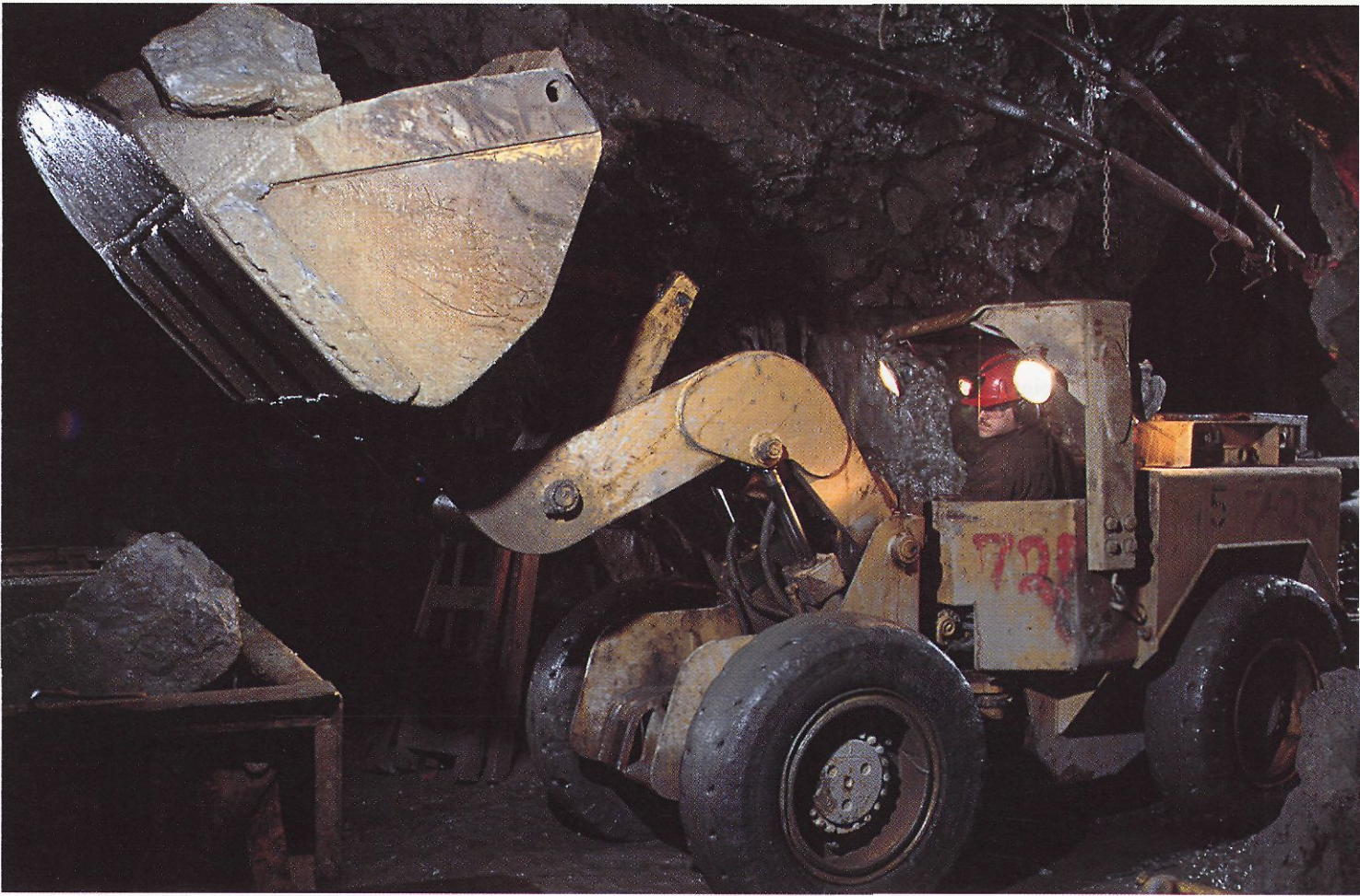
Load-haul-dump machine, Premier Gold Operations
