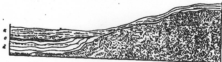
DIAGRAM REPRESENTING MODE OF OCCURRENCE OF GOLD. MISSION CREEK. a. Recent gravels. b. Crystalline rocks. c. Auriferous gravel. d. Tertiary deposits. e. Line representing present bed of stream.
