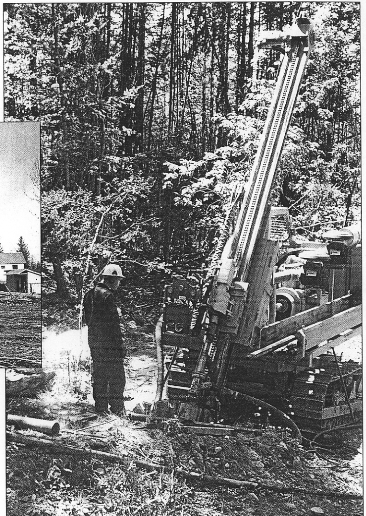
Reverse circulation drilling.
