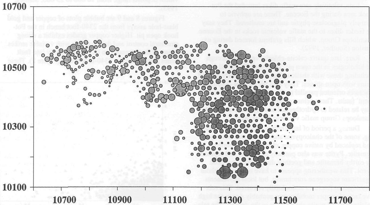
Figure 9. Bubble plot of production blast-hole gold assays from the 2340-foot bench of the Pothook open pit. Assays have been transformed and scaled to enhance geochemical contrast. The smallest and largest bubbles correspond to gold grades of 0.034 and 28.972 grams per tonne, respectively (n = 635).
