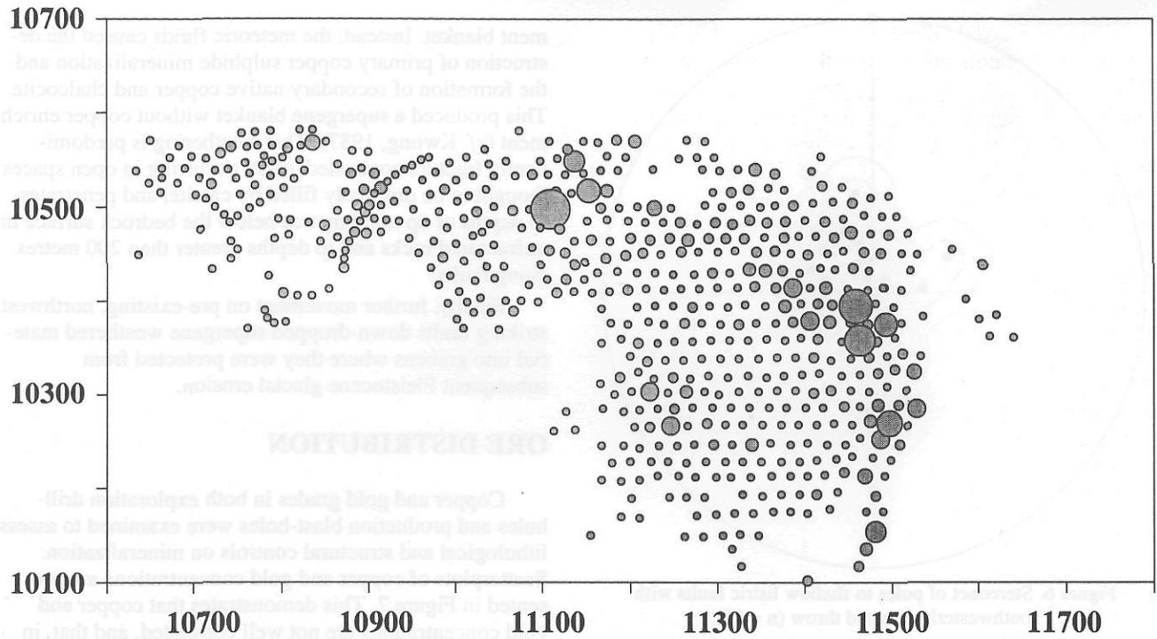
Figure 8. Bubble plot of production blast-hole copper assays from the 2340-foot bench of the Pothook open pit. Assays have been transformed and scaled to enhance geochemical contrast. The smallest and largest bubbles corresponds to copper grades of 0.01% and 2.60%, respectively (n = 635).
