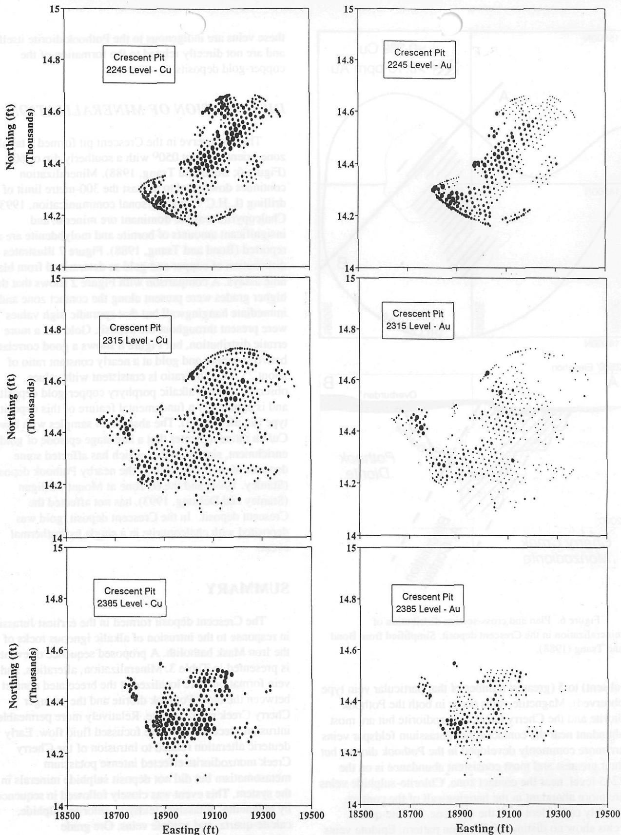
Figure 7. Bubble plots of copper and gold blast-hole assays. Data are shown for each of the four main benches. Bubble diameter is proportional to value. For each respective level N, the number of data points, maximum and minimum copper grade (wt. %), and maximum and minimum gold grade (g/t) are: 2175 level, 258, 2.09, 0.09, 0.82, 0.035; 2245 level, 349, 1.41, 0.06, 0.86, 0.00; 2315 level, 511, 1.83, 0.11, 1.82, 0.00; 2385 level, 236, 1.25, 0.13, 1.41, 0.035.
