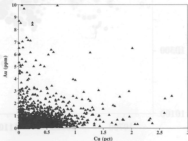
Figure 7. Scatterplot of exploration drill-hole and production blast-hole copper and gold assays from the 2100, 2160, 2220, 2280, 2340 and 2400-foot benches in the Pothook open pit ( $n = 3992$ ).
