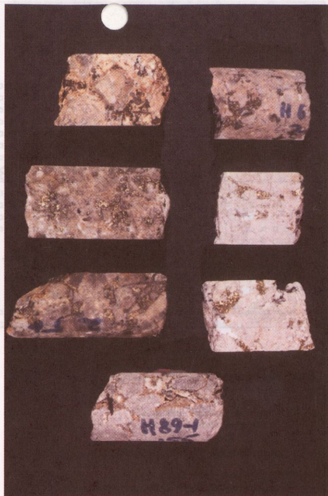
FIGURE 12. Typical drill core, Hearne Hill breccia pipe.
