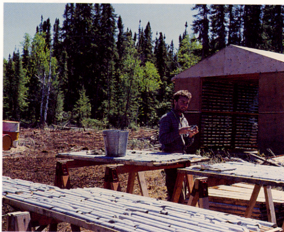
Core samples are laid out in the sunshine at the Little Stull exploration camp in northern Manitoba.
