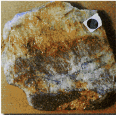
Molybdenite-bearing quartz stringers in granite porphyry from Max Property - (black circle is 1cm in diameter). Photo courtesy Roca Mines Inc.
