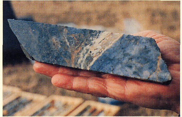
Core sample from Ann claim containing over 11 g/t gold
