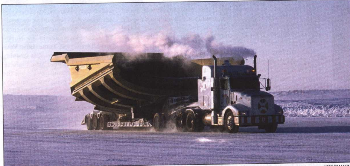
This past winter's shortened ice road season in the Arctic delayed the transport of large items, and forced De Beers to fly others in at Gahcho Kue at a higher cost. Here a 24-wheeler hauls a 200-tonne payload compartment of a much larger truck across a winter road to the Diavik diamond mine, 300 km northeast of Yellowknife, N.W.T. Diavik Diamond Mines is owned 40% by Aber Diamond Mines, with the remainder held by Rio Tinto.
