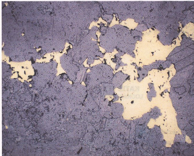
FIGURE 7. Chalcopyrite interstitial to carbonate-quartz alteration vein that cuts plagioclase-dominated andesite. Plagioclase is partly sericitized. DDH YKT-9239, 96.1 m depth. (I.L., x 2.5).
