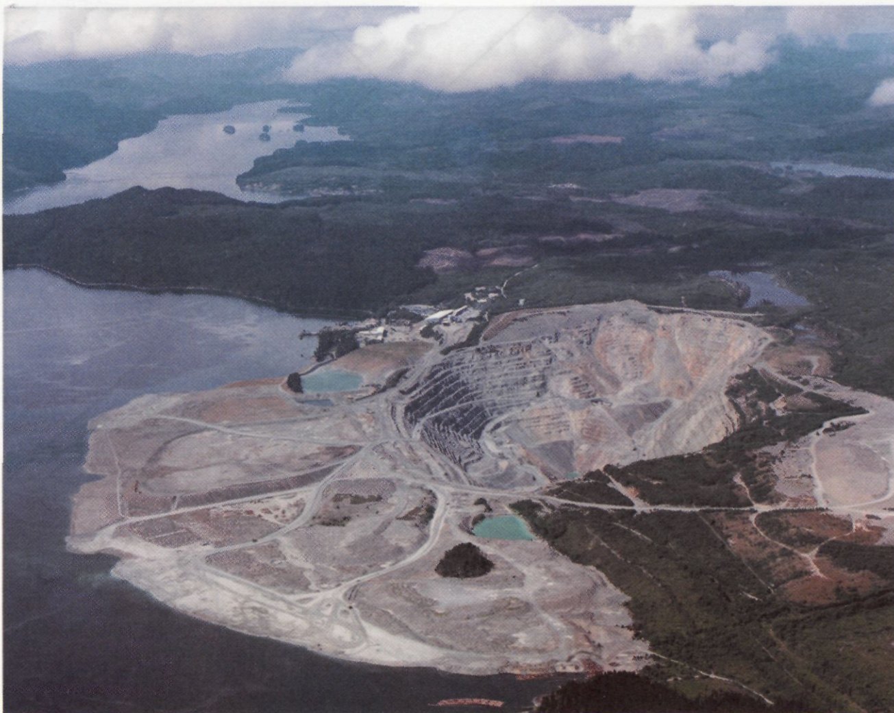
FIGURE 1. Aerial view (1993) of the Island Copper mine looking from above Rupert Inlet northwest across the open pit and plant site. In the foreground is Red Island surrounded by the marine waste dump. Bay Lake lies on the far side of the pit and Quatse Lake is in the distance. Holberg Inlet and the (unincorporated) municipality of Coal Harbour are visible to the upper left. In the pit, the End Creek Fault occurs as a dark trace down the south wall. The Pyrophyllite breccia zone lies at the west end of the pit between the fault and the talus slope in the middle of the far wall. The pit bottom is 340 m below sea level. The ultimate pit bottom will be 402 m below sea level, deeper than the surface of the Dead Sea (398 m below sea level), the deepest site on earth with direct sunlight.
