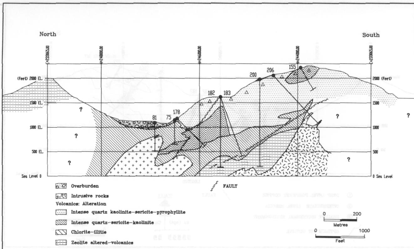
FIGURE 6. Section 233065 showing simplified geology, alteration and drillholes at Hushamu-McIntosh.
