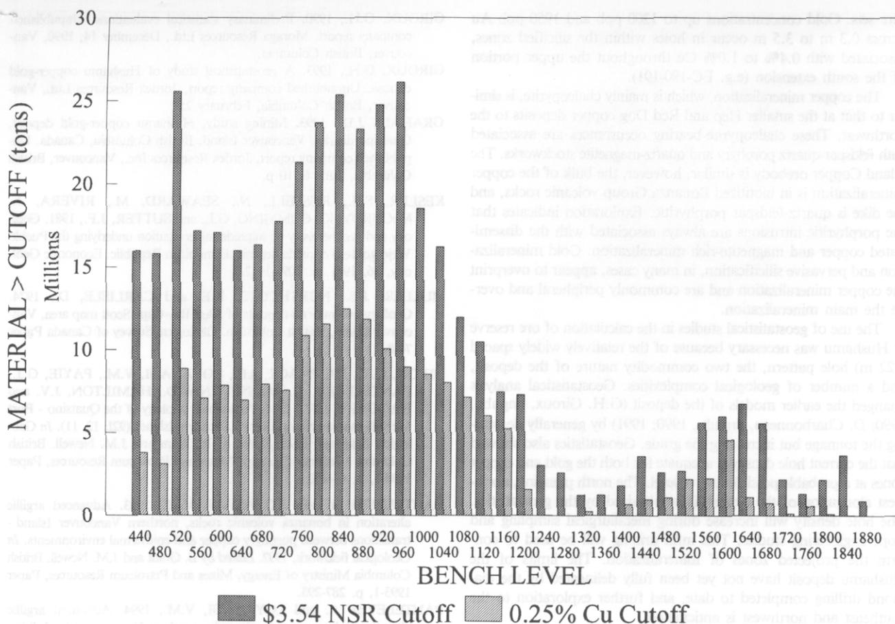
FIGURE 8. Geological reserves of Hushamu deposit showing tonnage by bench utilizing either a 0.25% Cu cutoff or a \$3.54 NSR cutoff (includes both copper and gold values and variable recoveries related to drill sample grade).
