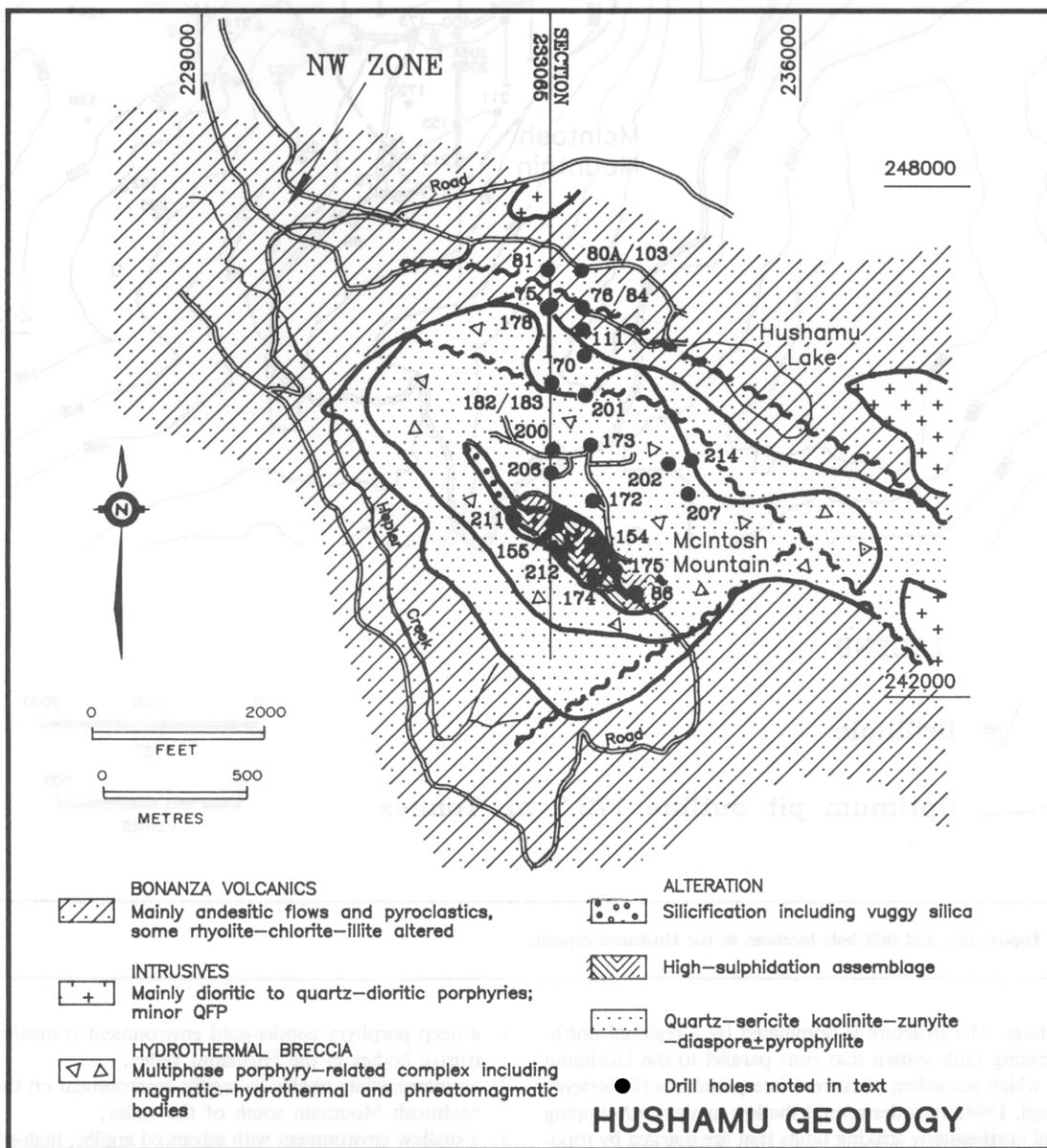
FIGURE 4. Simplified geological plan of Hushamu-McIntosh zone showing breccia complex and alteration. Inserts show extent of copper-gold geochemistry and ground magnetics anomalies.
