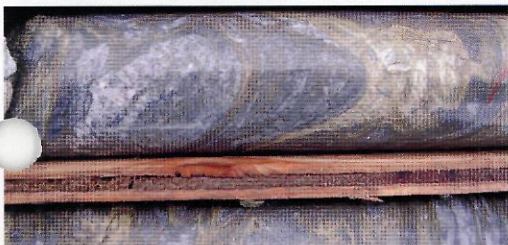
Banded semi-massive sulphide mineralization drilled in the area of the BRT Discovery Showing at
