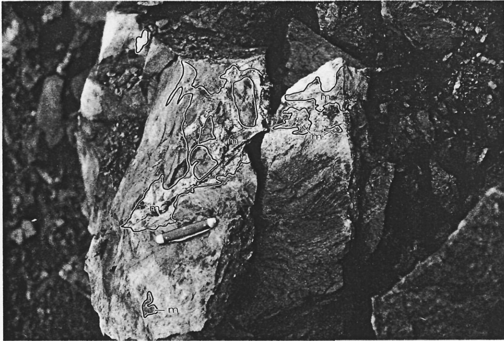
Plate VI. Broken molybdenum ore, Red Mountain mine, showing a variety of hornfelsic fragments; m indicates molybdenite.
