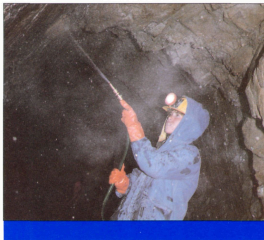
Howard vein material is washed prior to sampling. Grades have ranged up to .624 ounces of gold per ton along 100 feet of drift length. On the Congress property, underground exploration continued to locate high grade gold, particularly on the Howard zone.
