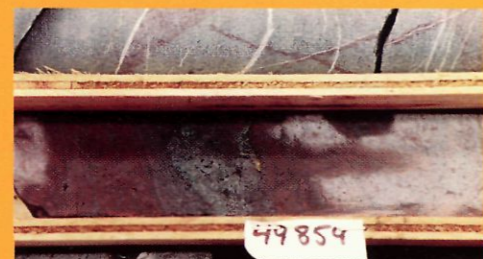
Section of hematite rich drill core with visible gold seen in the centre
