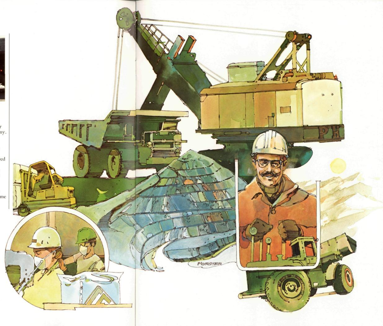
The "open pit" method of mining was selected as the best approach. The pit began in 1953 as a combination side-hill and mountain-top excavation. Over the years it has been progressively deepened to its present stage of development. Current production requirements call for mining some 1,300,000 tons of ore annually to produce more than 100,000 tons of asbestos fibre. To accommodate the "phase mining plan" some 6,000,000 cubic yards of waste rock are removed each year.
