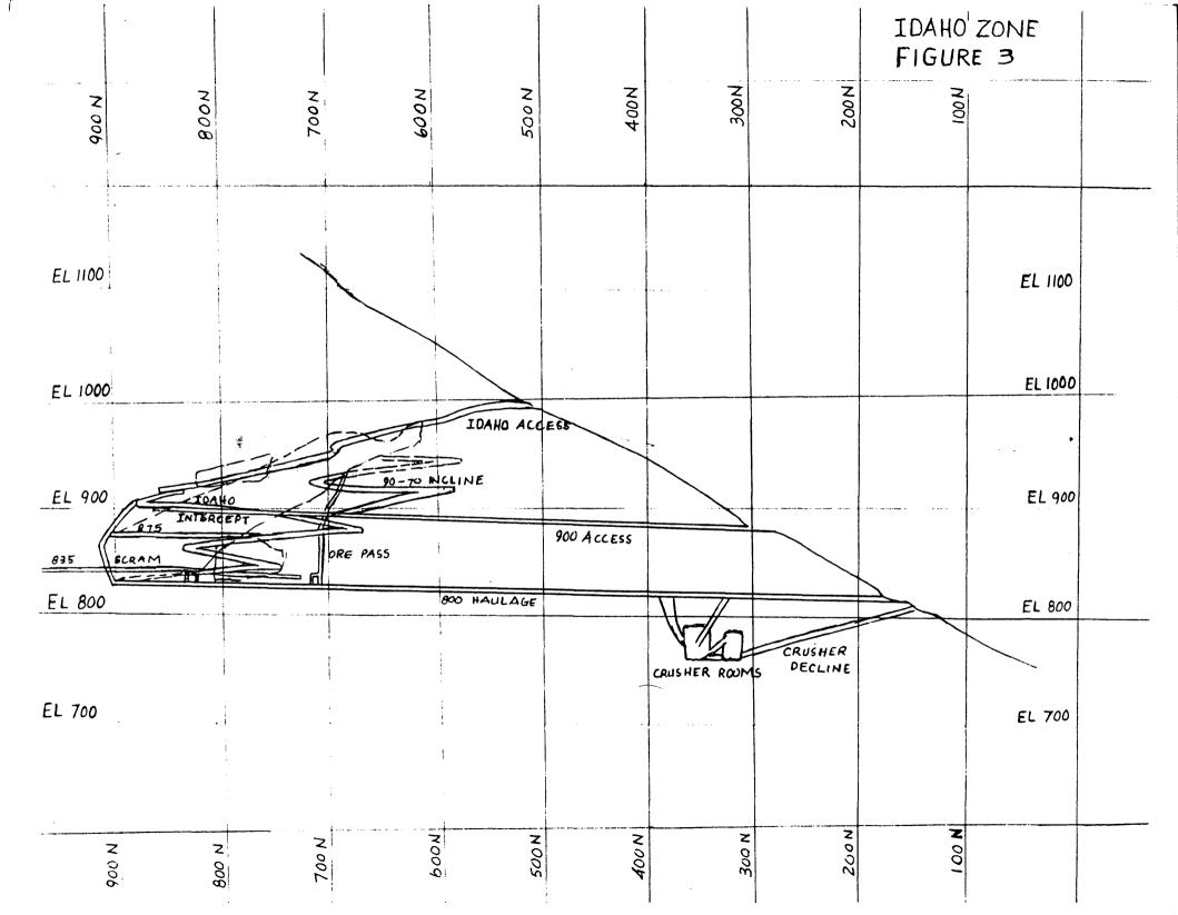
Due to the differences in size of the various lenses and their irregular wall outlines, it is not possible to introduce a standard stoping pattern. Each stope must be individually engineered.
