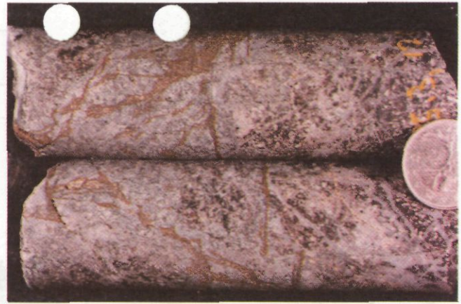
FIGURE 10. Pyrite veinlets with pale grey sericite envelopes cutting biotite-magnetite-hematite-sericite altered porphyry. Veinlet-controlled pyrite is the most widespread manifestation of phyllic alteration within the Red Bluff porphyry hydrothermal system. The sample is from Skyline drill hole S-1201 (105.3 m), drilled at the southeastern end of the porphyry.
