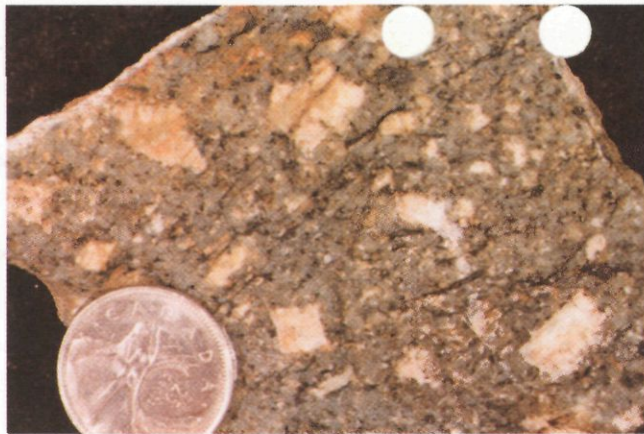
FIGURE 7. Sample from the Red Bluff porphyry collected near the base of the Red Bluff cliffs (Fig. 3). K-feldspar megacrysts and sericitized plagioclase phenocrysts occur in a saussauritized fine-grained matrix. The coin is 2.4 cm in diameter.
