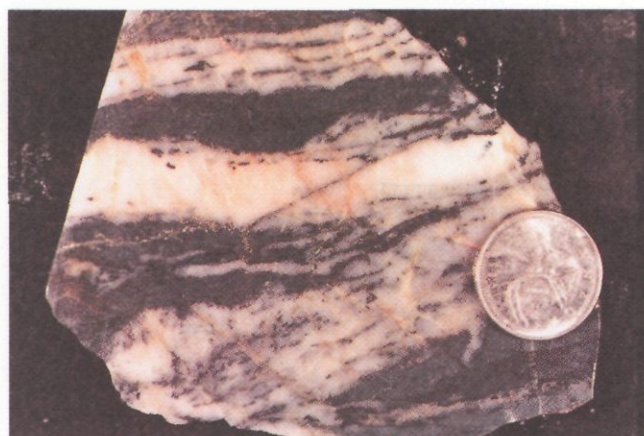
FIGURE 8. Sheeted quartz-magnetite-hematite veins with well developed magnetite + hematite laminae. The veins occur parallel to foliation in a strongly altered phyllitic matrix of dark grey sericite + magnetite + quartz + hematite + biotite. Sample is from the 130 portal at Snip (Fig. 5).
