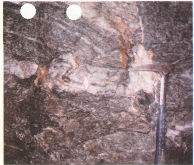
FIGURE 13. Sheeted foliation-parallel quartz veins with magnetite \pm pyrite laminae in a matrix of foliated K-feldspar megacrystic porphyry. Note the asymmetric S-shaped fold in the largest vein that suggests a normally-directed shear sense (top of photo to right). A late, thin milky quartz veinlet cuts the other veins and foliation beside the hammer. The view is looking southeast. The photo is from the Snip 130 portal.
