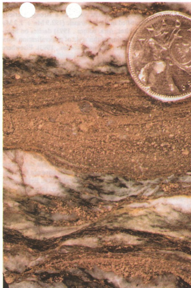
FIGURE 16. Twin zone sulphide and quartz ore types. Interlayered quartz, pyrite and quartz + calcite + chlorite veins. A synthetic shear band crosses the compositionally layered calcite + quartz + chlorite vein in the centre of the picture and indicates a left lateral apparent shear sense (top side to the left) which corresponds to an in situ normal sense of shear.
