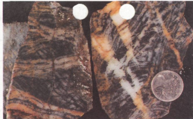
FIGURE 9. Intense quartz-magnetite-hematite veining. Multiple cross-cutting veins with abundant magnetite-hematite laminae comprise the entire volume of both samples. Younger veins have progressively less Fe-oxides. Both samples were collected from the base of the Red Bluff cliffs.
