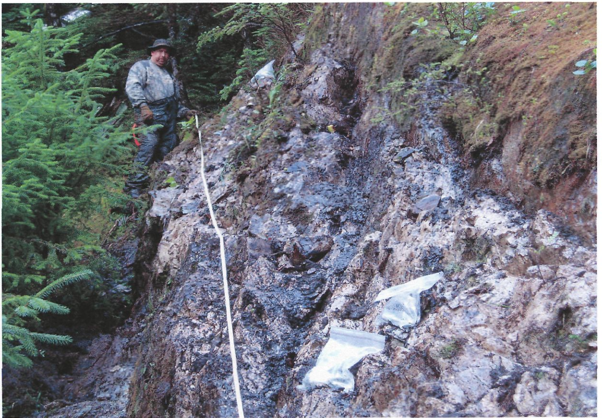
Photo 6 Discovery outcrop during sampling after shallow overburden hand stripped, tape measure is on left side of vein which is approx. 1.0m wide.
