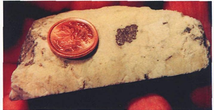
With a penny for scale, an unusually large crystal of pyrochlore can be seen. Pyrochlore is an oxide of sodium, calcium, niobium and tantalum. Most of the tantalum and niobium mineralization at the Blue River Project is on a much smaller scale. Photo by Ellsworth Dickson
