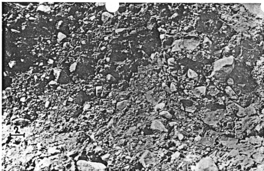
Figure 4. Example of unsorted, unstratified till at the Granisle Copper mine. Sub-rounded to angular cobbles and pebbles are enclosed in a fine silty clay matrix. The width of the picture is approximately 1 metre
