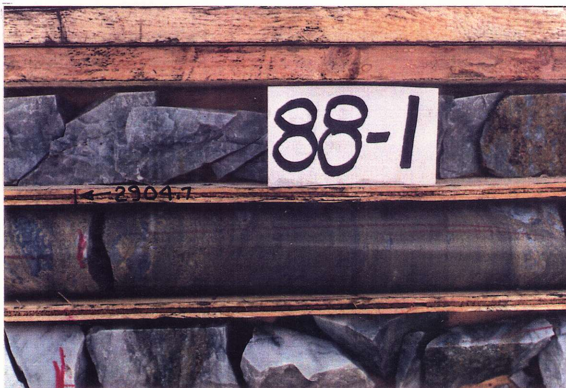
Hole 88-1 Sphalerite showing banding at 2904.7'
