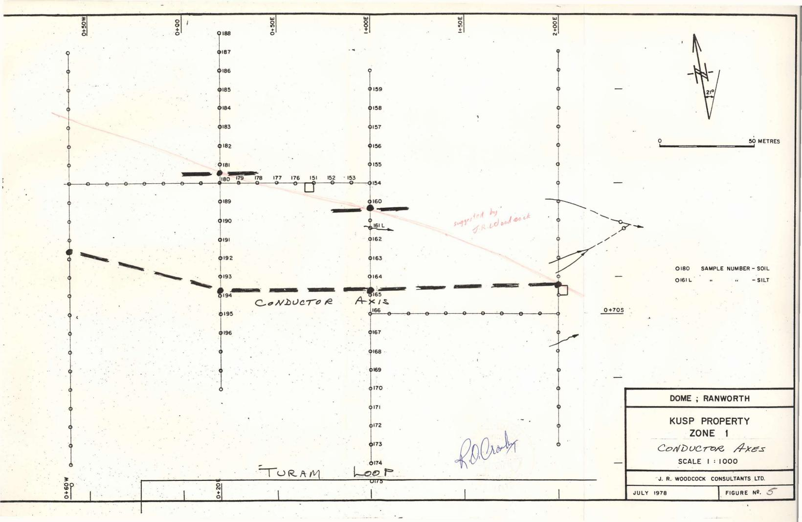
Line 1+00 E was completed at both 400 and 800 Hz. The higher frequency yield better results, so lines 2+00 E and 0+20 E were surveyed at 800 Hz.
