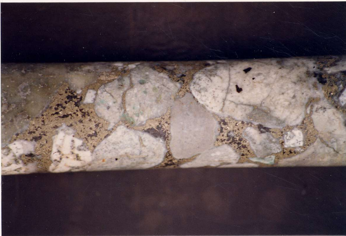
PLATE 1 - Stockwork pyrite, sphalerite, galena mineralization from TR 88-4. Interval (706.8 ft. to 710.1 ft.) assayed 0.383 oz/T Au.
