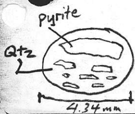
fig 1 - elongate pyrite frags in Qtz.
