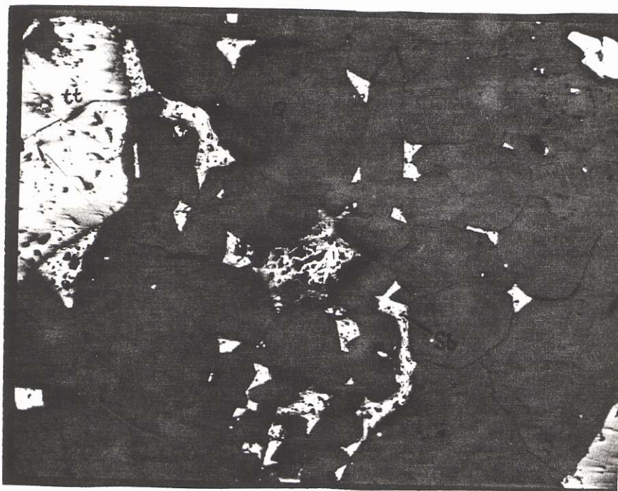
(Photomicrograph 1) Photomicrograph of euhedral quartz (dark), with fine grained interstitial stibnite (sb), needles. Note the tetrahedrite (tt), also with minor interstitial stibnite. (Planed polarized light, 56X, V-10)
