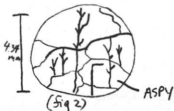
(Fig 2) Depiction of fractures branching in arsenopyrite grains
