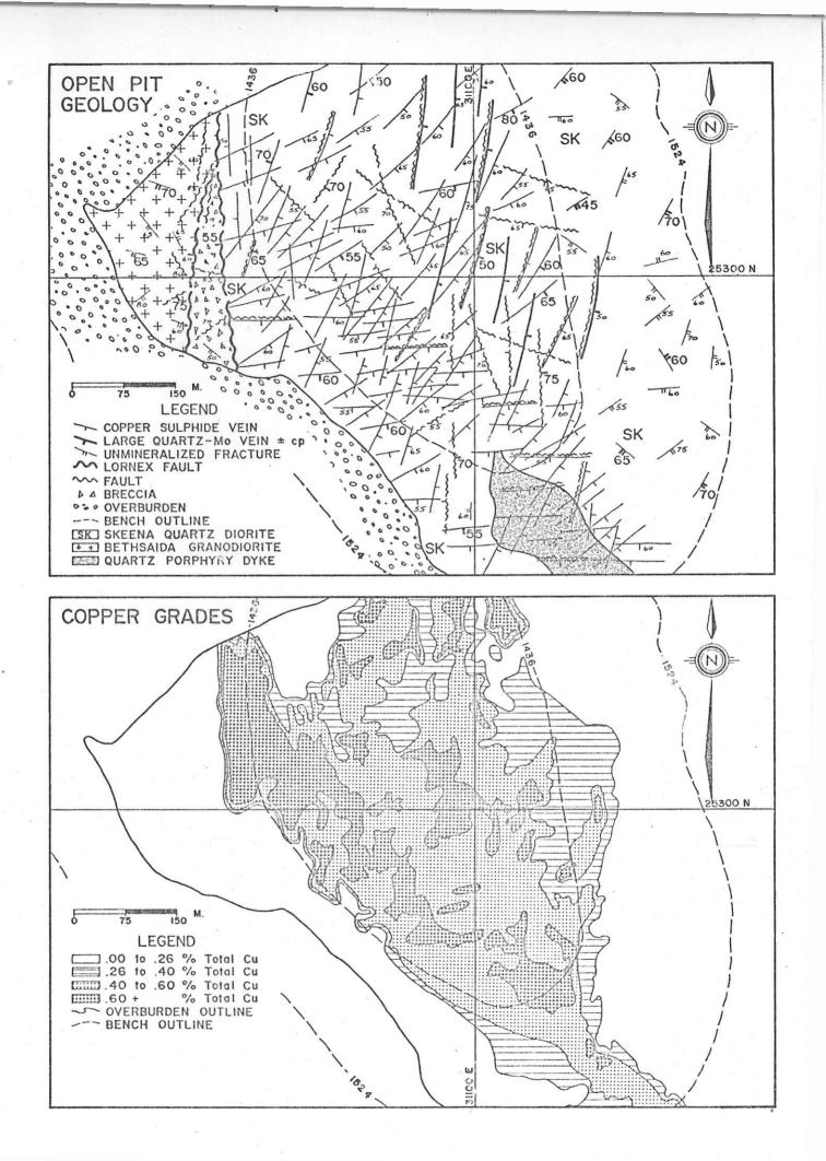
Tectonic stresses (maximum principal stress from NE and SW) develop vertical conjugate shears and related extension fractures at the intersection of the north striking Lornex fault and the northwest trending quartz porphyry dyke. (Stippled area is region of most intense fracturing).
