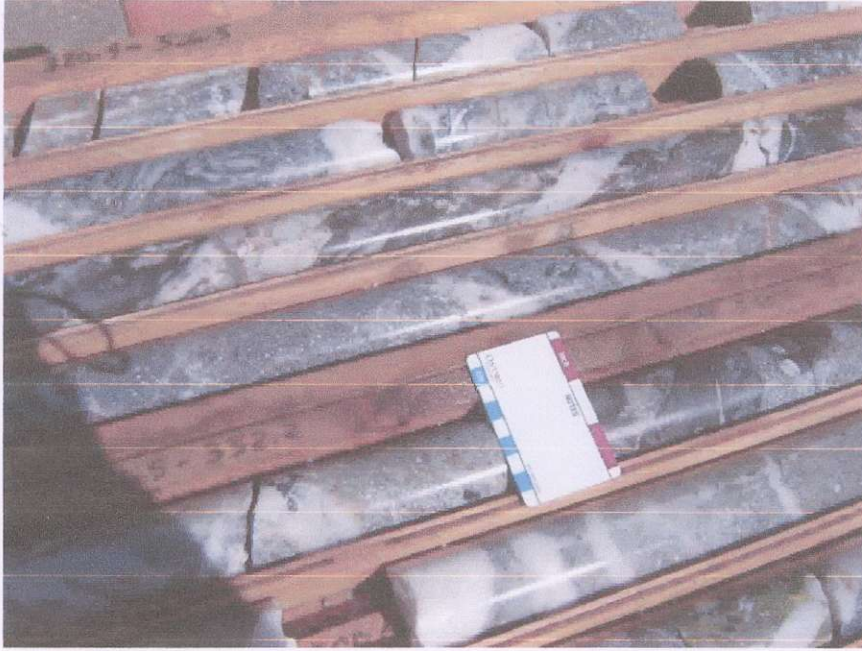
Photo 1 - Hole MM04-01 – Intermineral granodiorite porphyry dyke with angular 1 – 3 cm fragments of Lardeau Gp country rocks and cut by at least 2 generations of weakly mineralized quartz veins
