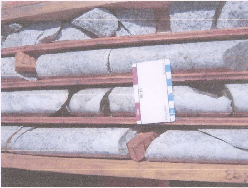
Photo 4 – Hole MX07-03 – Weakly mineralized leucocratic, altered (bleached) granodiorite separating two intervals of quartz vein-hosted, high grade Mo mineralization near bottom of hole. Note quartz eyes immediately right of top end of scale.
