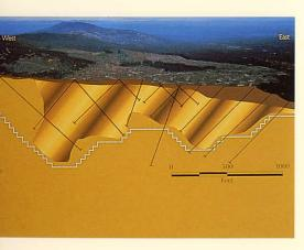
An immense, 6 square mile, gold-copper rich sulphide system exists around alkalic monzonite stocks which intrude volcanic strata. Drilling of 315,000 feet in 406 holes within the eastern portion of this system has confirmed two major bulk tonnage gold-copper deposits and numerous high grade gold veins. The balance of the sulphide system and other targets on the 21 square mile joint venture property remain to be drill tested.
