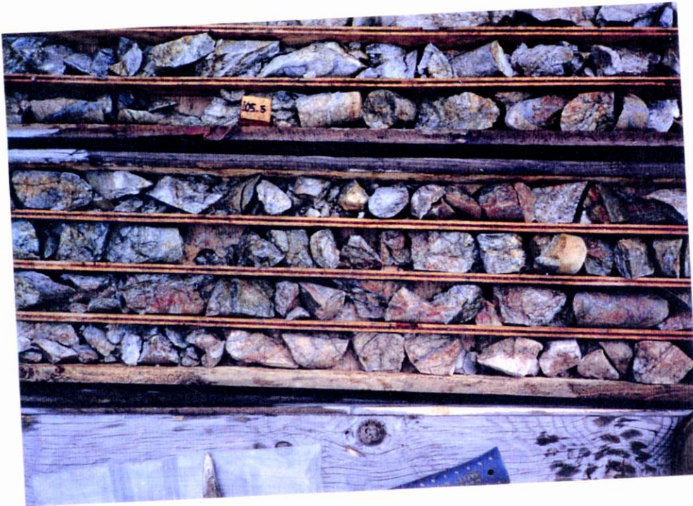
Core from Corona drill hole 89-18 - includes part of better mineralized section at end of hole (94.6-121 metres - 26.4 metres - 0.41% copper, 0.012 oz/ton gold).
