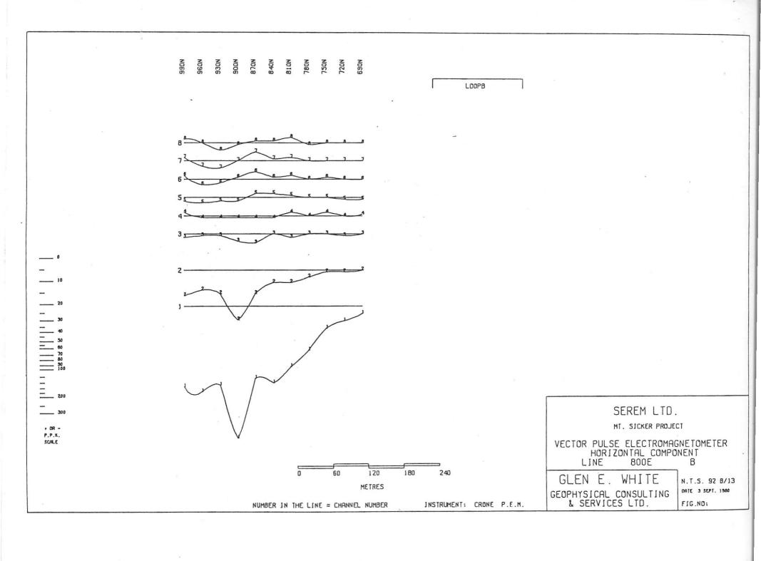
840. 780% LOOPB SEREM LTD. MT. SICKER PROJECT + OR -P.P.K. VECTOR PULSE ELECTROMAGNETOMETER VERTICAL COMPONENT SCALE 800E LINE В 120 180 GLEN E. WHITE N.T.S. 92 B/13 METRES DATE 3 SEPT. 1980 GEOPHYSICAL CONSULTING & SERVICES LTD. FIG.ND: INSTRUMENT: CRONE P.E.M. NUMBER IN THE LINE = CHANNEL NUMBER
