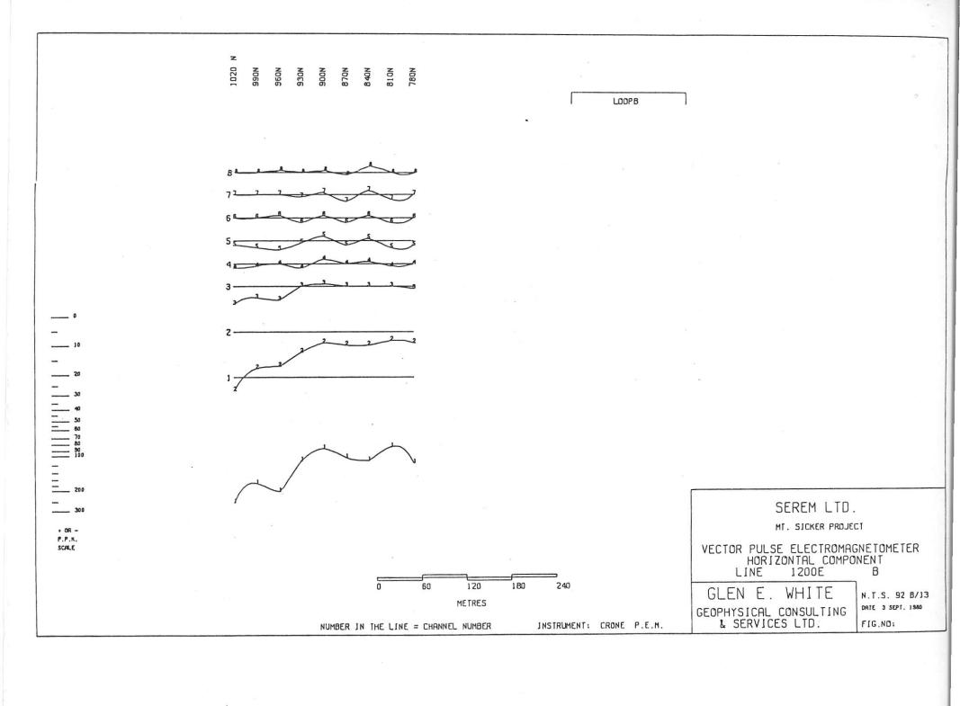
900N LOOPB SEREM LTD. MT. SICKER PROJECT VECTOR PULSE ELECTROMAGNETOMETER VERTICAL COMPONENT + OR -P.P.K. SCALE В LINE 1200E GLEN E. WHITE 180 240 120 N.T.S. 92 B/13 DATE 3 SEPT. 1980 GEOPHYSICAL CONSULTING & SERVICES LTD. METRES FIG.NO: INSTRUMENT: CRONE P.E.M. NUMBER IN THE LINE = CHANNEL NUMBER
