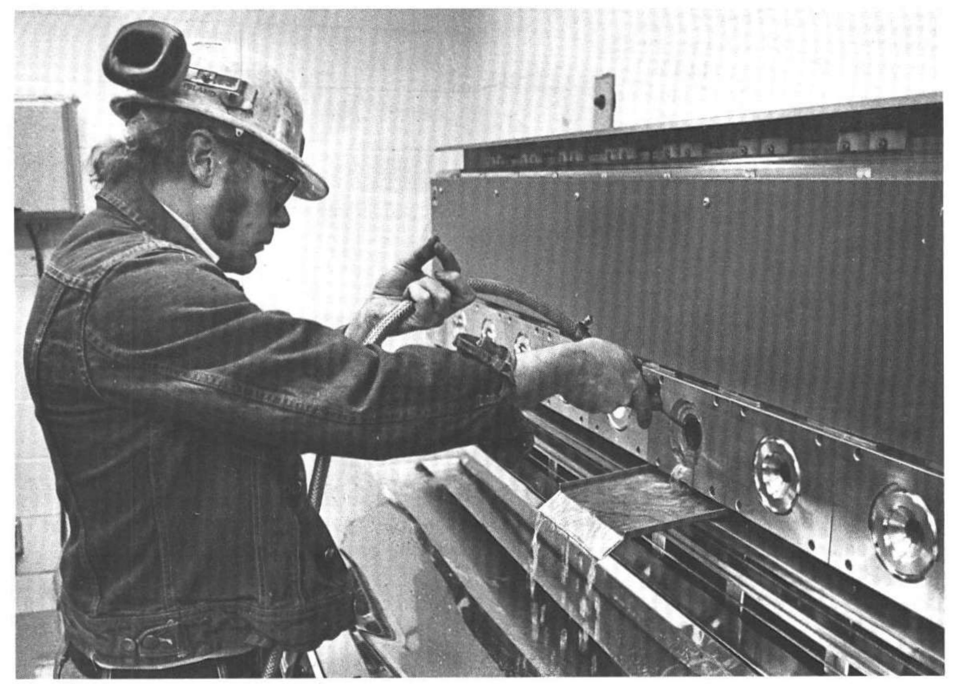
An on-stream analyzer in the mill at Island Copper provides computer printouts on the recovery and quality of the various products.
