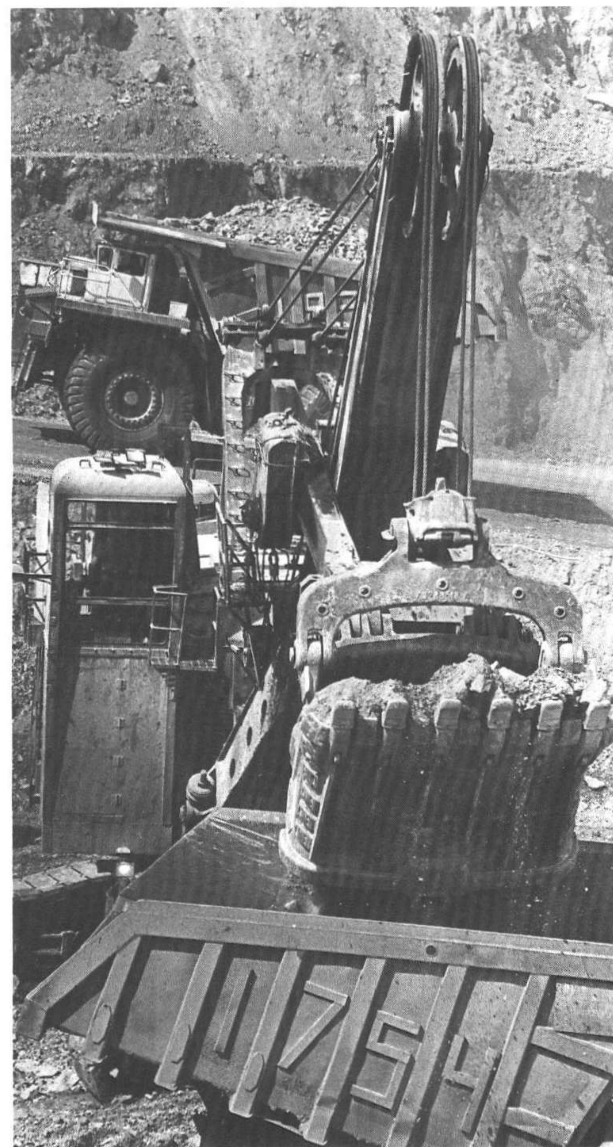
Electric shovels can load 120-ton and 170-ton capacity trucks in minutes, ready for transportation to the crusher.
