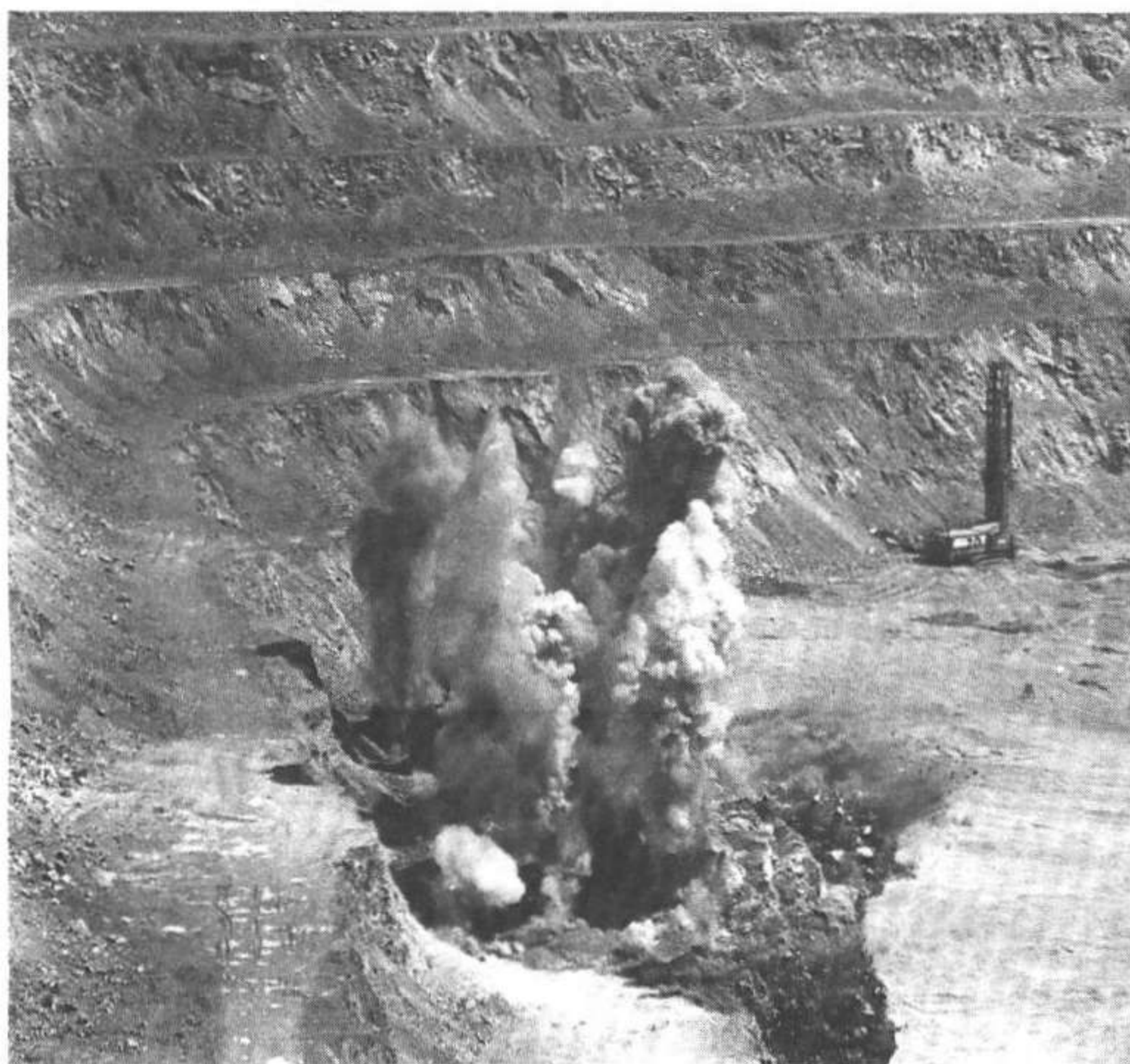
Blasting in the pit is a sophisticated daily process to expose the ore first discovered by prospectors such as Gordon Milbourne.
