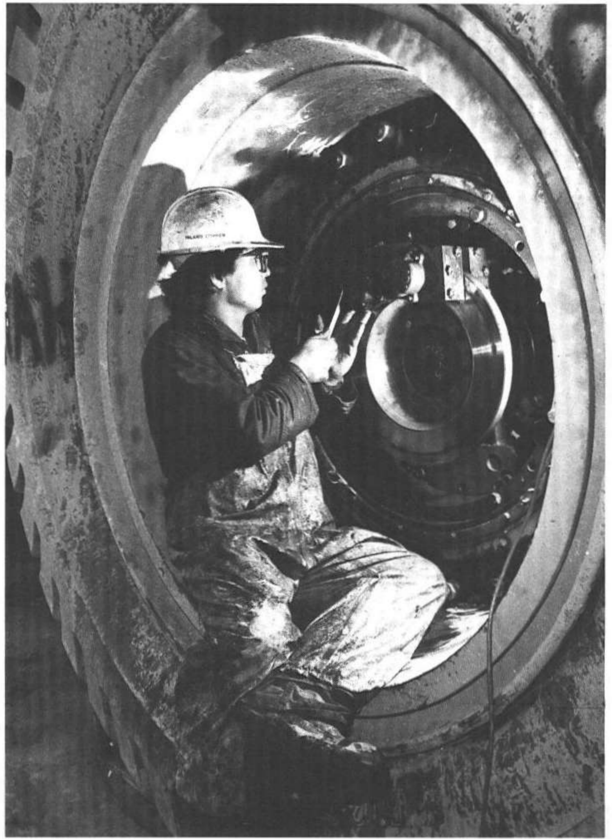
Close-up view of an Island Copper mechanic working on the wheel of a giant haul truck.
