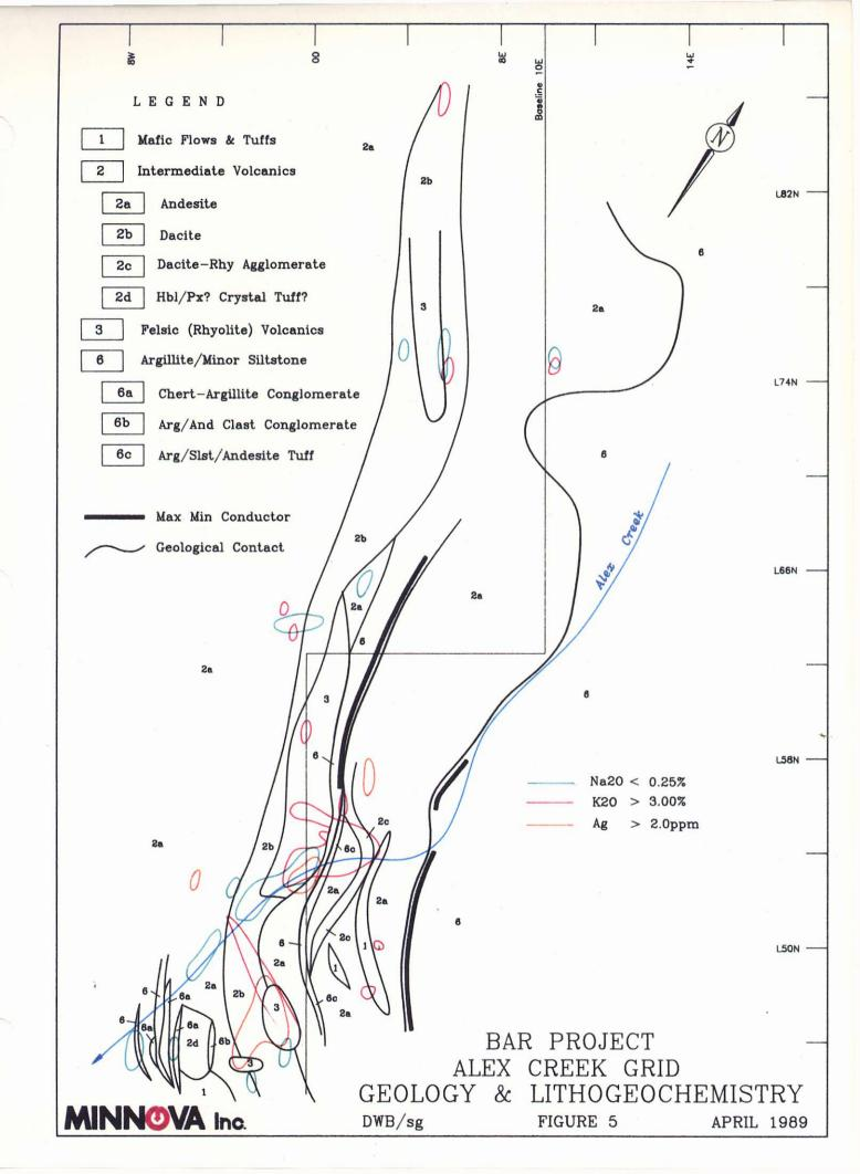
strongest mineralization in the area occurs in Alex Creek near the south end of the grid where intermediate volcanics contain up to 20% stratiform pyrite over a width of about one metre. Significant base metal sulphide mineralization was not detected, although minor amounts of malachite occur locally with pyritic intermediate volcanics. A quartz vein containing 1% chalcopyrite and 2-4% malachite occurs in an altered andesite just off the grid at about L65N.
