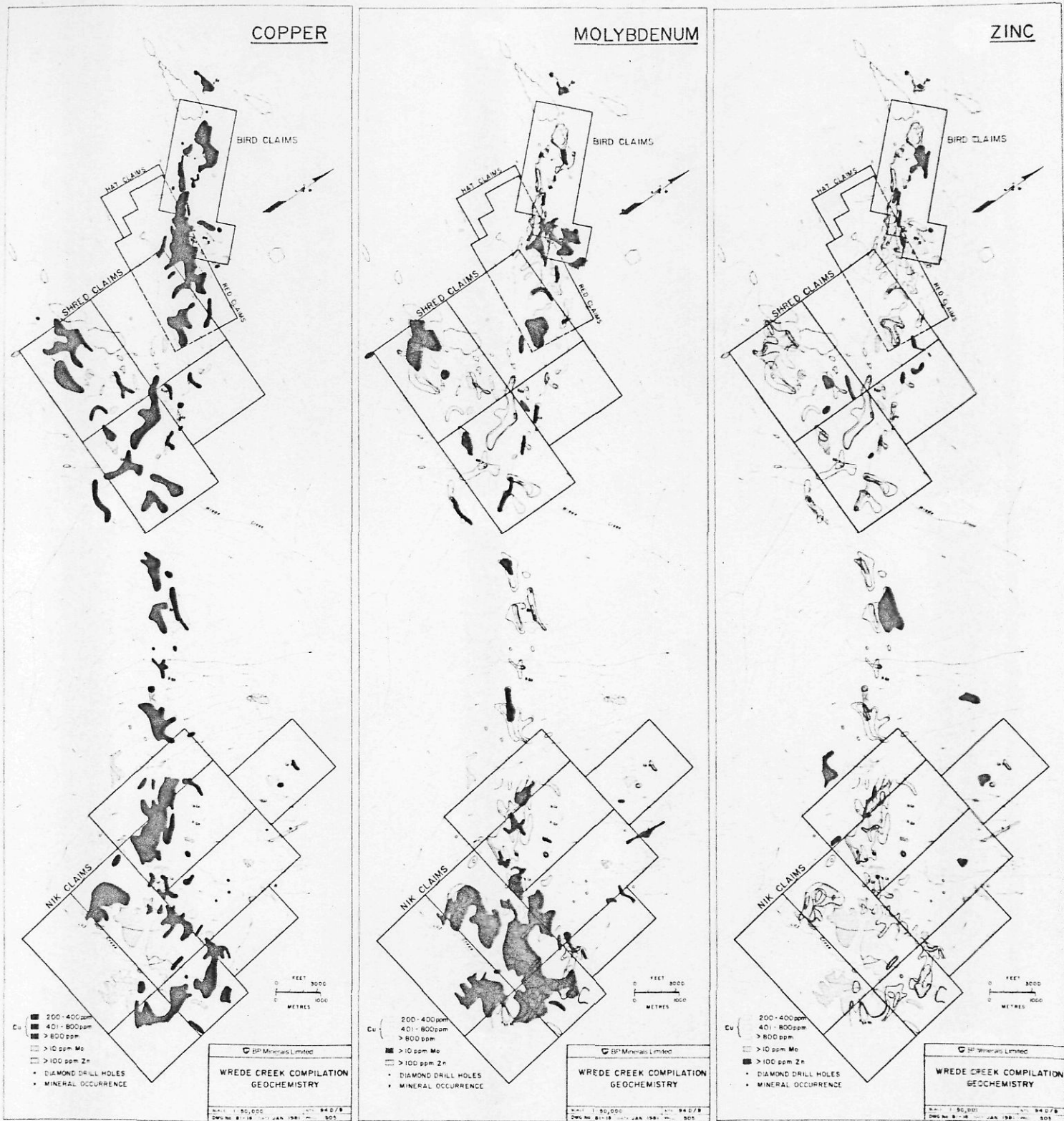
Figure 2: Wrede Creek compilation geochemistry Copper, molybdenum and zinc content of soils and talus fines.
