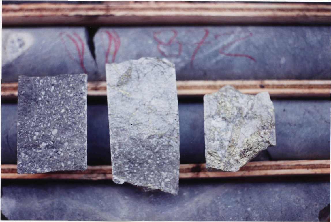
Mineralization: Biotite feldspar porphyry (left). clay-sericite alteration front with cpy veining (centre) high grade cpy stockwork (right)
