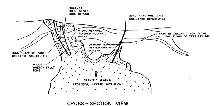
Figure 1. Generalized geological map and cross-section views of typical bonanza gold-silver lode deposits, western Nevada (modelled after Comstock Lode).
