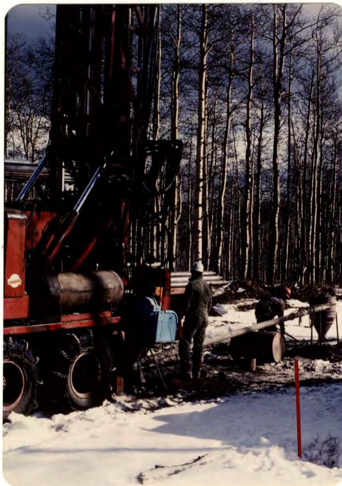
Drilling was completed using a truck-mounted T985H Schramm Hammer Drill. A cyclone was used for catching samples.
