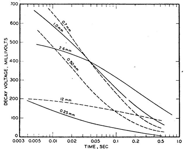
Fig. 4—Observed decay voltage  $e(t)$  as a function of time. For  $V = 15$  volts,  $v = 0.02$  and  $\sigma = 5 \times 10^{-3}$  mhos/m. This graph and Fig. 5 are examples of extensive overvoltage experiments at Newmont's laboratories in Jerome, Ariz. Fig. 4 illustrates work in transient domain, Fig. 5 work in frequency domain.
