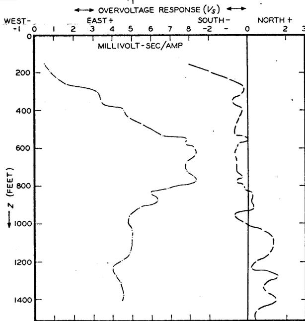
Fig. 12—Nababeep West, South Africa, borehole WP 12. The direction of mineralization from a drillhole is indicated here by the overvoltage azimuth survey.
