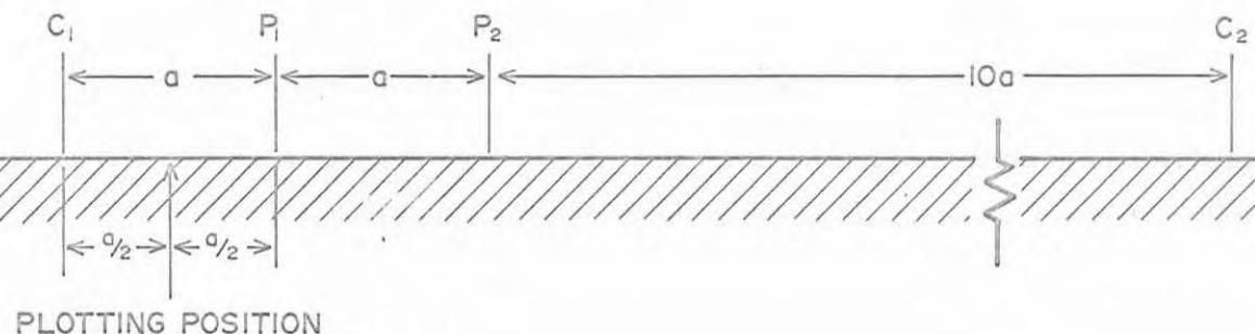
FIG: 2 POLE-DIPOLE ELECTRODE CONFIGURATIONS.
