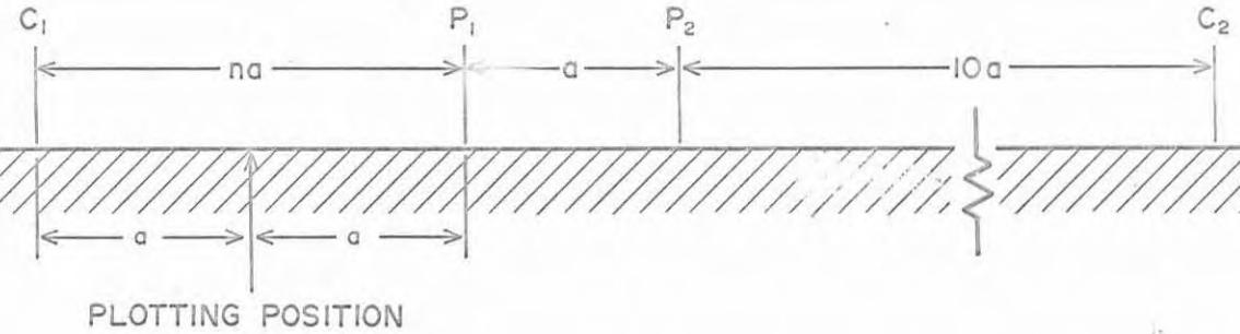
EQUISPACED THREE ELECTRODE ARRAY
