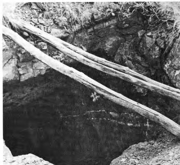
Porcupine shaft. Depth 70 feet on a high grade copper zone.
