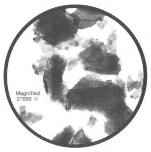
The plate like particles of AlSi Mica viewed through a super magnifying electron microscope
