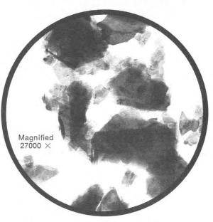
The plate like particles of AlSi Mica viewed through a super magnifying electron microscope
