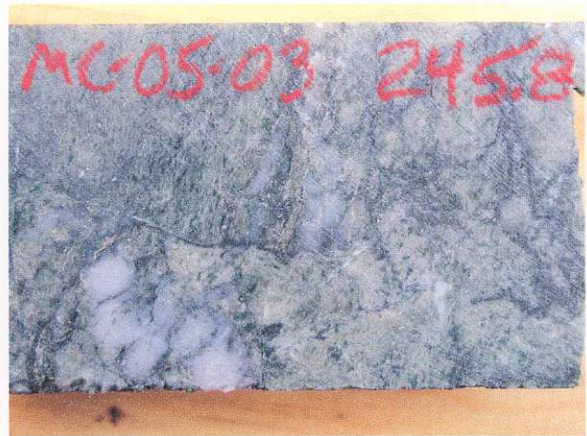
MC-05-03 245.8m Phyllic altered hydrothermal breccia beneath Sulphurets fault
