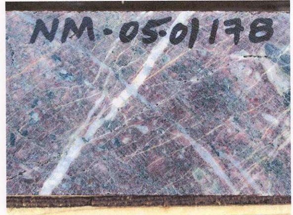
NM-05-01 178m Propylitic-potassic altered, veined granite porphyry
