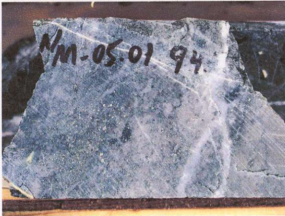
NM-05-01 94m Silicified, veined andesite
