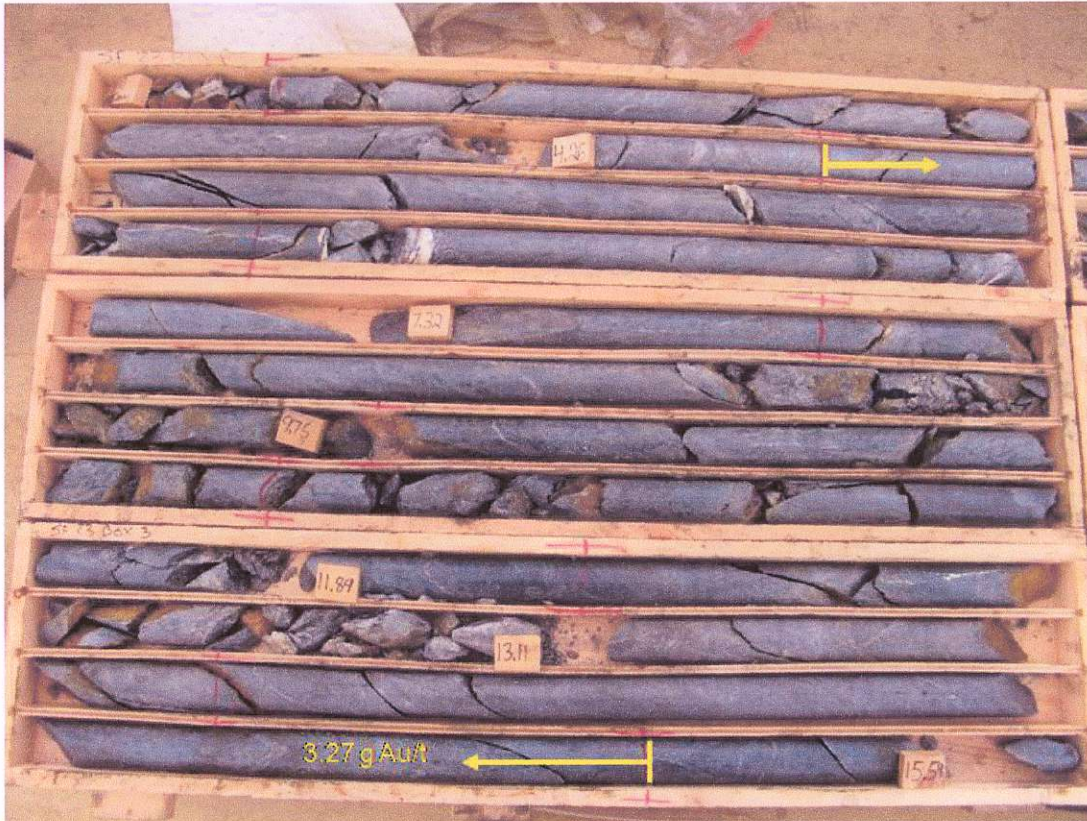
Photograph 7: Mineralized drill core from DDH SF-23; marked intercept from 4.57 to 15.24 m. (Modified after Burk, 2007)
