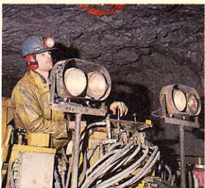
A "jumbo" drill used for underground work - advancing the decline, drifting and crosscutting.
