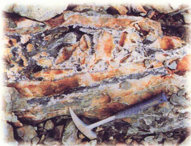
Vuggy quartz vein/breccia with vein of grey, massive specular hematite. Typical of high sulphidation epithermal precious metal deposits.
