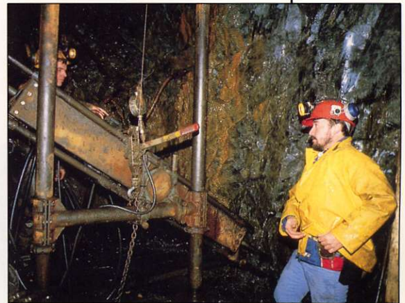
Underground diamond drilling
