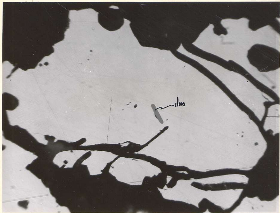
Figure 2 Mag. 316x. Photomicrograph of a polished section of py (pale grey) containing small inclusion of ilm (dark grey) in gangue (black).
