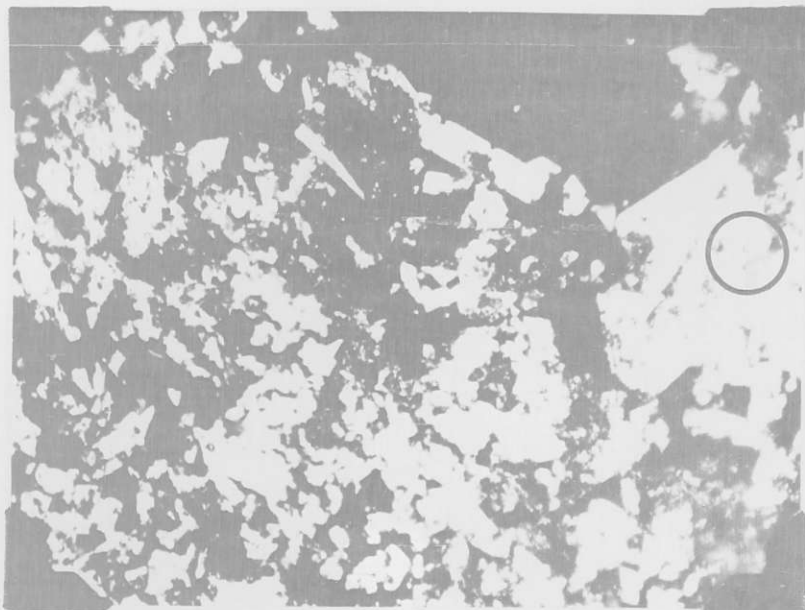
Disseminated Arsenopyrite and Pyrite. 875 X. Note grey mineral veining pyrite. (In circle)
