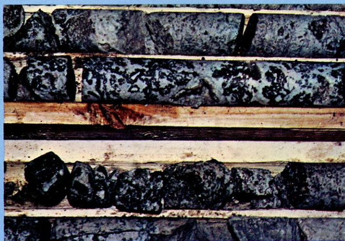
Core from hole no. 25 of the Great Slave Reef Project assayed 22.52% of combined lead and zinc over a length of 17 feet.
