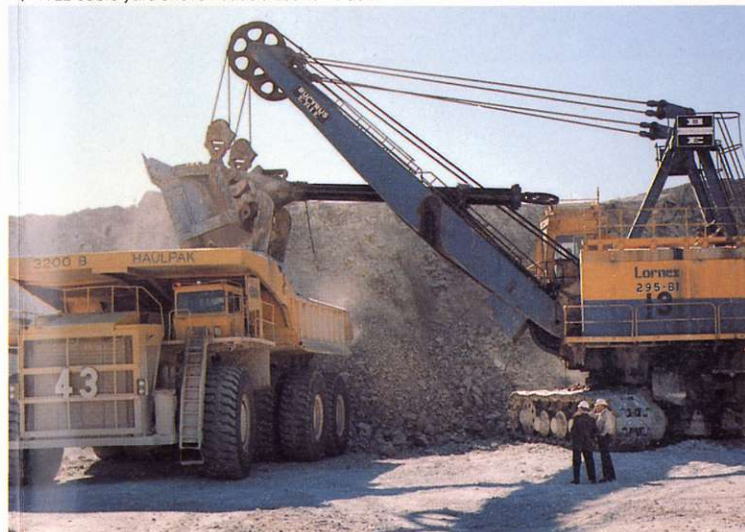
▼ A 22-cubic-yard shovel loads a 235-ton truck
